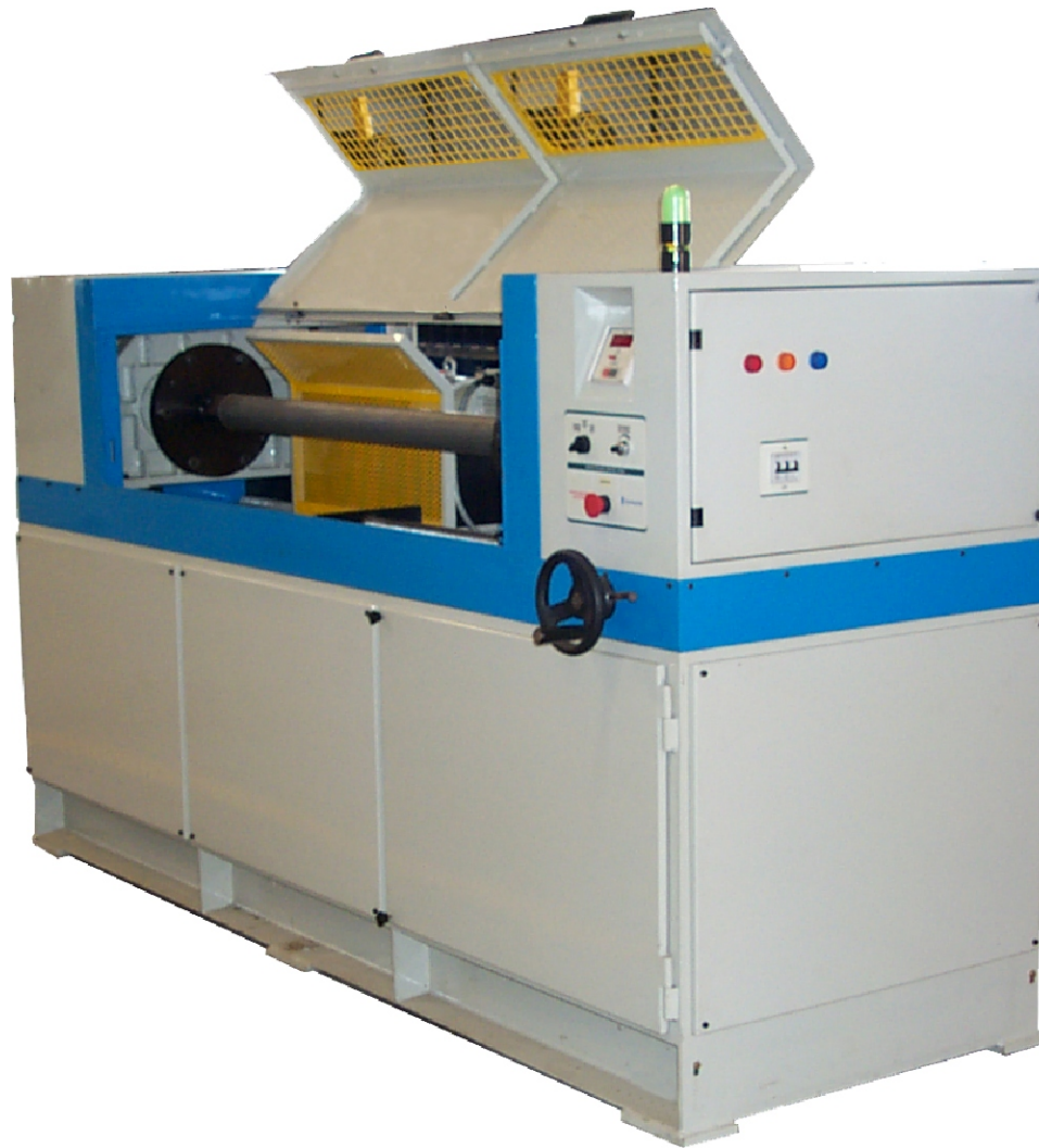
Test Rig for testing the torsional strength of Propeller Shafts
