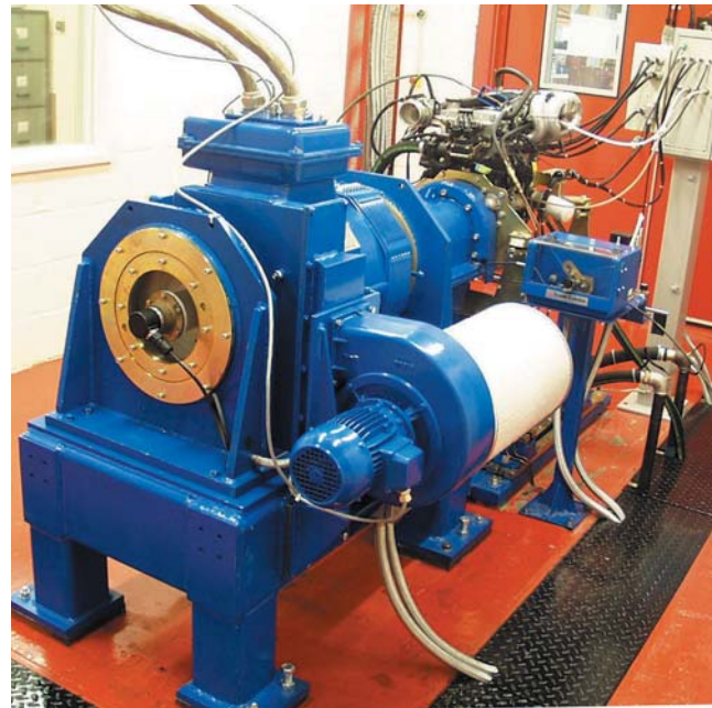
Typical engine test installation
